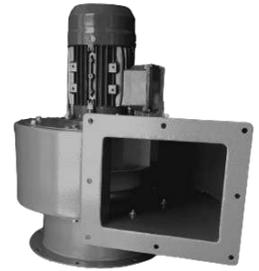
Equipped with a snail-shaped scroll without support, the RSH vertical fan is directly mounted for operation with a vertical shaft. Compact, it is perfectly suited for installation on the roof of any industrial equipment requiring the extraction of hot and/or dusty air, such as paint booths.
