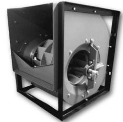
Equipped with a double-inlet backward impeller, the RDH fan is compact and highly efficient. It is used in various applications such as ventilation, air conditioning, and cooling systems. Designed for belt-driven transmission, it offers multiple operating points.
