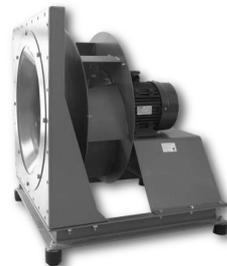
Without a scroll, the RLM fan is particularly suitable for free discharge. It integrates easily into systems with limited space, such as plenums, booths, and air handling units. It adapts to the existing structure and is generally used in round or rectangular enclosures.
